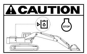
7) HYDRAULIC OIL LUBRICATION(Item 8) This warning label is positioned on the right side of air breather.
